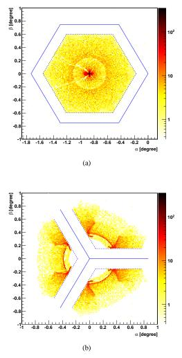
Fig. 5. The spot seen at the PMTs. Lines are drawn to represent the pixel boundaries (solid) and the light guides boundaries (dashed). Photons simulated with the expected position at the pixel centre (a) and at the vertex of the light guide (b).
