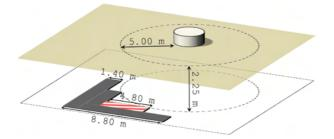
Fig. 2: Schematic view of one possible arrangement of the AMIGA detector pair consisting of one SD station and four buried muon scintillation counters. The hatched module with a length of 4.8 m will be used for the first prototype.
