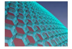
Fig. 2. View of the camera in the Geant4 simulation. The picture show the light guides in light blue and the PMT windows in red.
