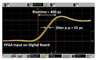
Fig. 7: Measured signal jitter.
