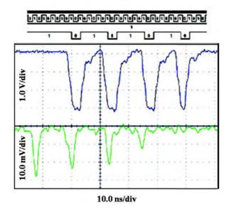
Fig. 4: Example of measured input and output pulses of the DB. The lower graph schows the amplitude of the input pulses, the middle graph the comparator output and the two upper graphs the clock and the resulting digital data in the FPGA.
