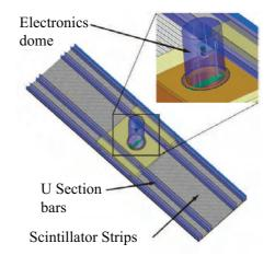
Fig. 2: AMIGA scintillator module. Top PVC panels covering the scintillator strips are not shown. High-lighted are the strips, the PVC U bars, the PMT and electronics dome, zoomed in the top right insert.
