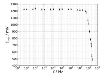
Fig. 5: Bandwidth measurement of a typical DB channel.
