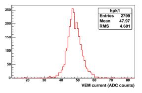
Fig. 2: VEM measured for 2799 PMTs.
