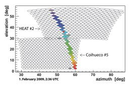
Fig. 3. This shower was recorded by HEAT telescope #2 and Coihueco telescope #5.The relative arrival time of the fluorescence light is coded in the colour of the pixel. The solid line is a fit of the shower detector plane.
