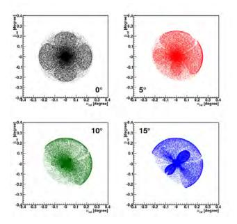
Fig. 4. Spots produced at the ideal focal surface for incident angles of  $0^{\circ}$ ,  $5^{\circ}$ ,  $10^{\circ}$  and  $15^{\circ}$ . For each generated photon the relative position ( $\alpha_{\mathrm{rel}}, \beta_{rel}$ ) with respect to the expected position for an ideal optical system is shown.
