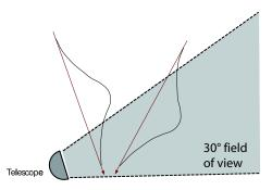
Fig. 1. Effect of limited field of view on reconstruction: Showers approaching the telescope have much higher reconstruction probability than those departing.
