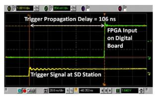
Fig. 6: Measured trigger propagation delay.
