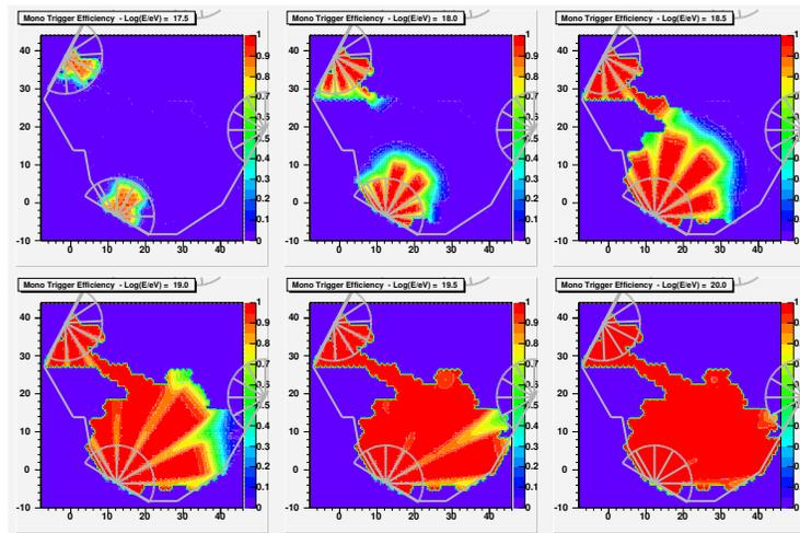
**Figure 3.** Mono hybrid trigger efficiency at mid October 2004, for proton primaries in ‘‘clean’’ atmosphere, at energies from  $10^{17.5}$  to  $10^{20}$  eV. Efficiency is represented following a color code from violet (0) to red (1). At this date, the two central telescopes (3 and 4) of both eyes were equipped with corrector ring lenses. The unusual shape of the domain where efficiency is greater than 0 is caused by the extent of the SD array at this date.
