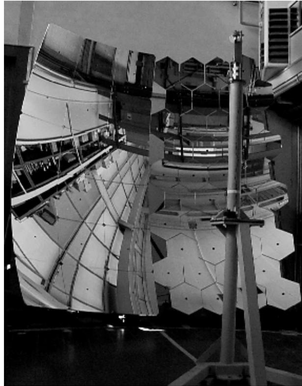
Fig. 3. Picture of the first telescope mirror. In this provisional mounting the aluminum mirrors (square shape) are combined together with the polished glass mirrors (hexagonal shape). The system for alignment is also visible on the front.
