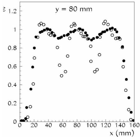
**Fig. 7.** The light collection efficiency was measured for a row of three adjacent pixels with (full points) and without (open points) the light collectors.
