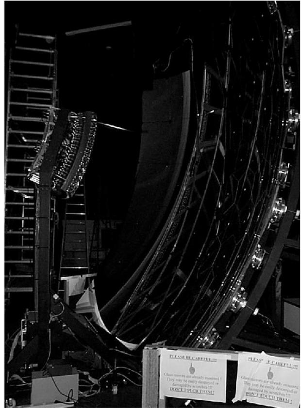
**Fig. 8.** The first fluorescence detector telescope assembled in the building of “Los Leones” on the Observatory site in Argentina. The camera on its support faces the mirror which is visible on the right side.
