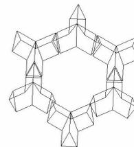
**Fig. 6.** Sketch of the light collector for one pixel. The six "mercedes" stars are arranged to form a hexagon.
