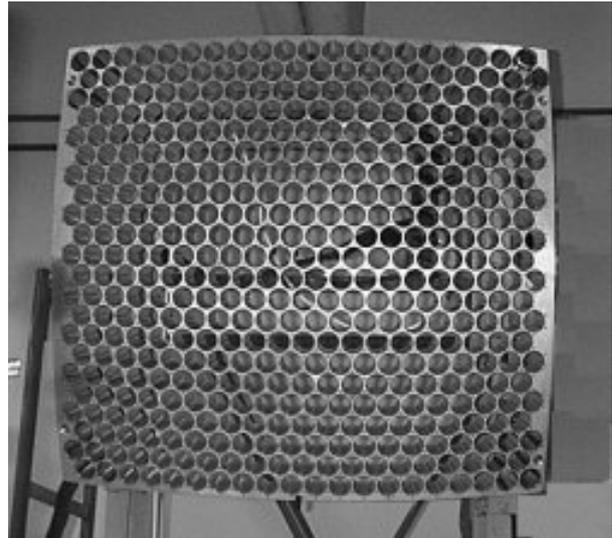
**Fig. 5.** Front picture of the camera body. The photomultipliers are inserted inside the cylindrical holes of the aluminum block.
