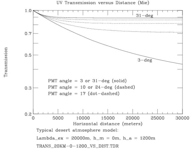
**Fig. 2.** Transmission factor,  $T^a$ , for Mie scattering on aerosols in the atmosphere. The aerosols are described by a horizontal extinction length,  $\Lambda^a(360nm) = 20km$  and an exponential scale height,  $h_a = 1200m$ . Curves are shown for Auger fluorescence telescope viewing angles from  $3^\circ \sim 31^\circ$  to the horizon.
