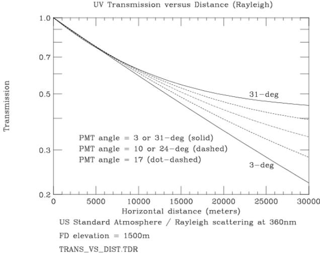
**Fig. 1.** Transmission factor,  $T^m$ , for Rayleigh scattering on the molecular atmosphere. Curves are shown for Auger fluorescence telescope viewing angles from  $3^\circ \sim 31^\circ$  to the horizon.
